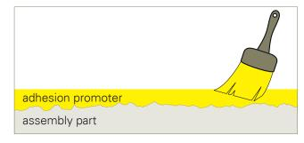
When the solvent evaporates, the adhesive / sealant can moisten the surface completely. Air pockets are prevented and the contact area is increased.
